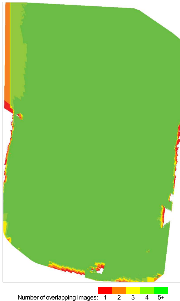
Figure 4: Number of overlapping images computed for each pixel of the orthomosaic. Red and yellow areas indicate low overlap for which poor results may be generated. Green areas indicate an overlap of over 5 images for every pixel. Good quality results will be generated as long as the number of keypoint matches is also sufficient for these areas (see Figure 5 for keypoint matches).
