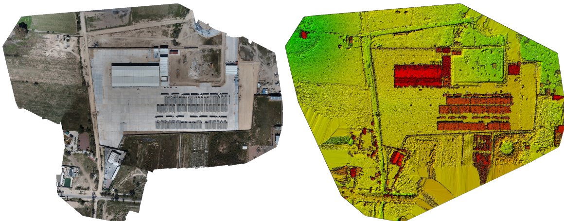
Figure 1: Orthomosaic and the corresponding sparse Digital Surface Model (DSM) before densification.
